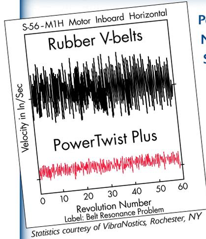
PowerTwist Plus, NuTLink and SuperTLink do not have the continuous tension cords found in conventional V-belts. As a result, transmitted vibration in the drive system can be reduced
