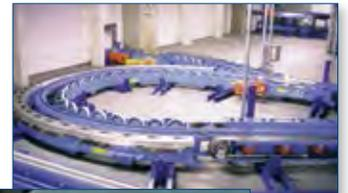
**Solution** *Roller drives were converted to run SuperTLink Wedge Belts. Not only did SuperTLink handle the drive misalignment with ease, system noise was reduced by 40% compared to the earlier chain-driven set up.*
