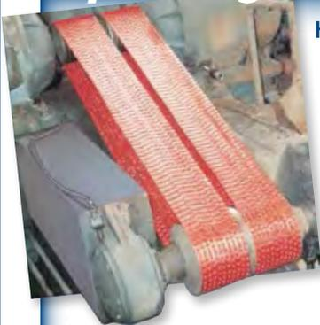
HPC V-Belts are manufactured from high performance polyurethane/polyester composite materials which ensure excellent durability even in the most demanding conditions. HPC V-Belts from Fenner Drives will
