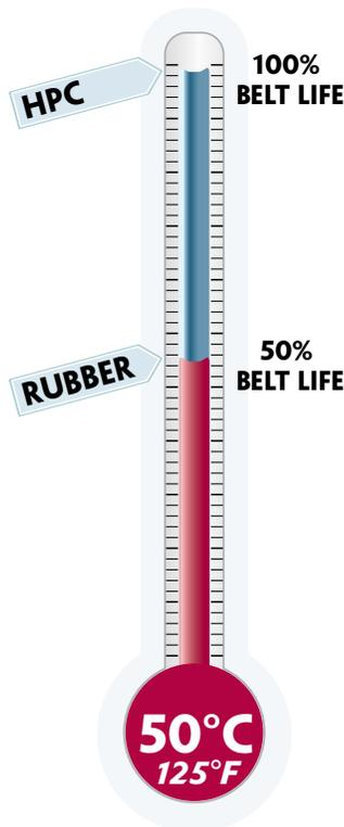
Fenner Drives HPC V-Belts are different in two significant ways. First, they are made of custom reinforced polyurethane elastomers with excellent resistance to high operating temperatures. Second, the unique link design results in belt constructions which limit flex induced heat build-up; a greater surface area also dissipates any heat generated more effectively as compared to a solid construction rubber V-belt... a lower internal belt temperature = a longer belt life.
