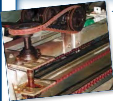
The unique link design of Classical and SP rated HPC V-Belts allows designers considerable freedom in their choice of optimum drive configuration with savings in component
