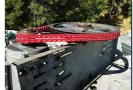
**Solution** On upgrading to PowerTwist Plus V-Belts, the maintenance team now carries boxes of the red belt 24/7. Drives are now serviced quickly without wasting time returning to the belt crib to pick up specific belt sizes. Stock was reduced to just a few boxes of 3L, A/13 and B/17 sections.
